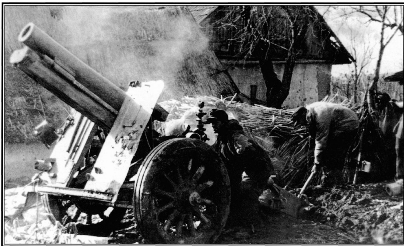
Above: A 15cm (5.87in) heavy artillery piece in action in East Prussia. The sIG 33 was one of the Germans' most powerful and reliable infantry field howitzers, but was difficult to manoeuvre due to its heavy weight.
