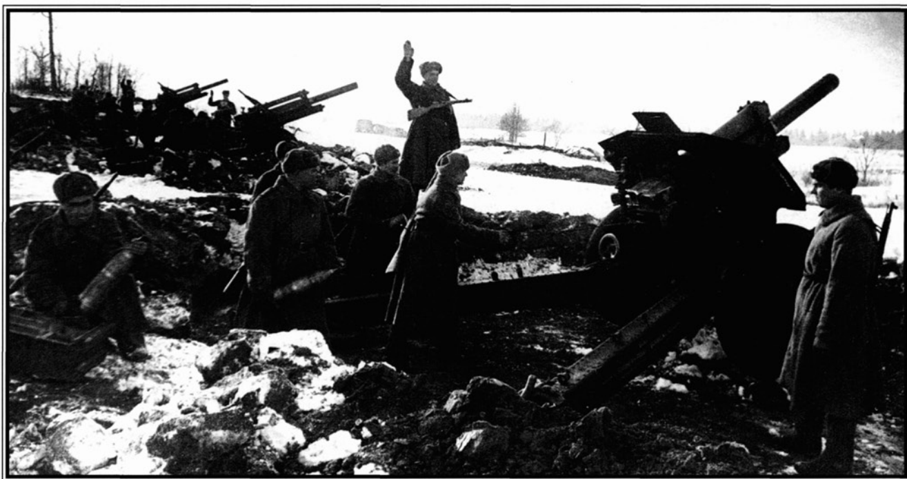
Above: The 76mm (3in) gun was the backbone of Soviet field artillery. Small enough to allow relatively easy mobility and use in a variety of types of terrain, the 76mm still had a range of roughly 12km (7.5 miles).
